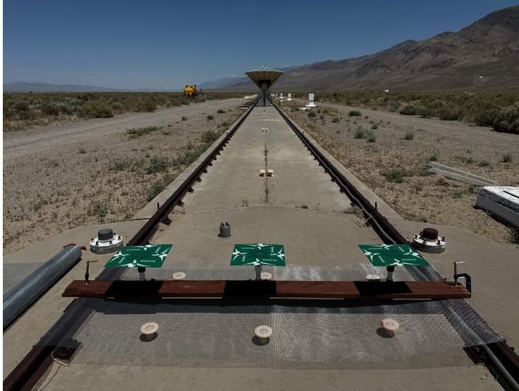
Figure 4.25: Test deployment of CASM-256 antennas and ground plane at the array site, the old railroad track in the middle of the DSA-110 array at Owens Valley Radio Observatory.
