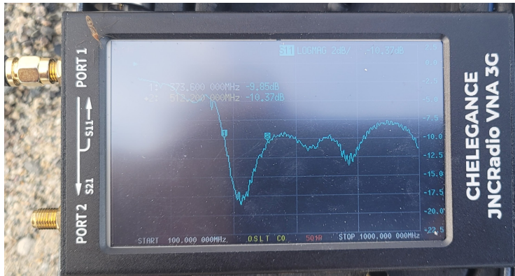
Figure 4.26: NanoVNA readout of a CASM-256 antenna prototype on a ground plane at Owens Valley Radio Observatory. Frequency range shown is 100 MHz to 1000 MHz. The reading confirms that the antenna has S_{11} < -10 dB for frequencies 375 - 500 MHz.
